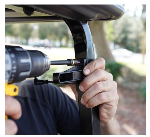
Press down on the topside of the bracket to keep the base flush with the frame when inserting the bottom screw
