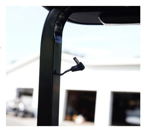
\*There are 2 white dots on the power cord. This mark indicates the minimum amount of cord length to leave outside the frame (a little longer is ok but shorter will not reach the power input on the unit)
