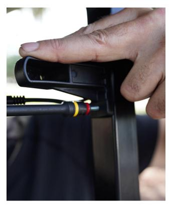
Insert power cord end into outside bracket hole to prevent length from being pulled down the frame when locating power cord in next step
