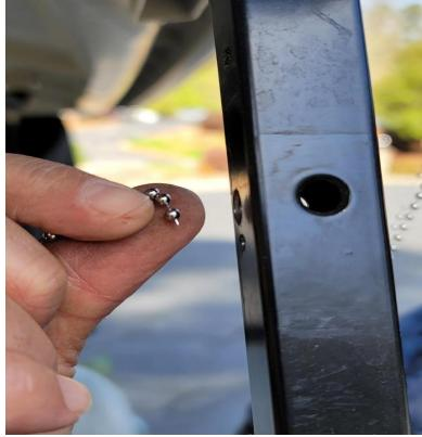
Using a paper clip, fashion a hook to "fish" or pull chain out of exit hole
