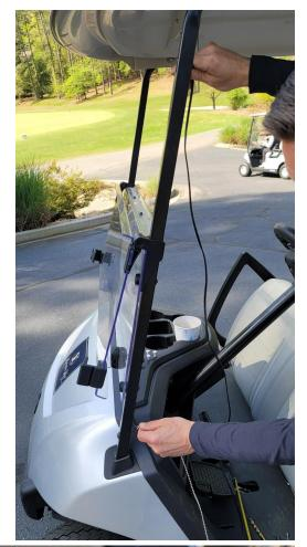
There is a white mark on the power cord four (4") from the plug. This mark indicates how much cord length to leave outside the frame (a little longer is ok but shorter isn't)
