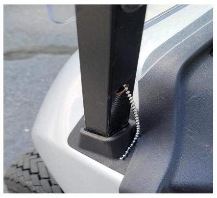
\*Hold the plug-end length of cord level, or above the entry hole when pulling from the bottom. This helps reduce damage to the cord that may result in grounding issues when connected to power
