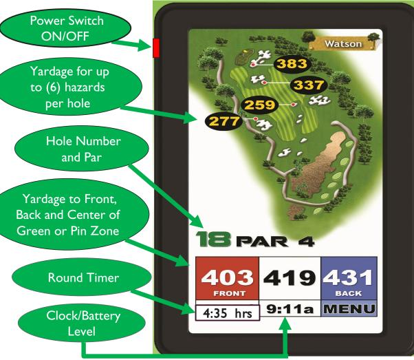
Charging Port is located on the back of the iPar7B. Turn the red power switch OFF(0) when charging. Green light on iPar charger indicates when battery is completely charged. To maximize battery strength...*turn it ON* when you leave the house, turn it OFF when you leave the course.
